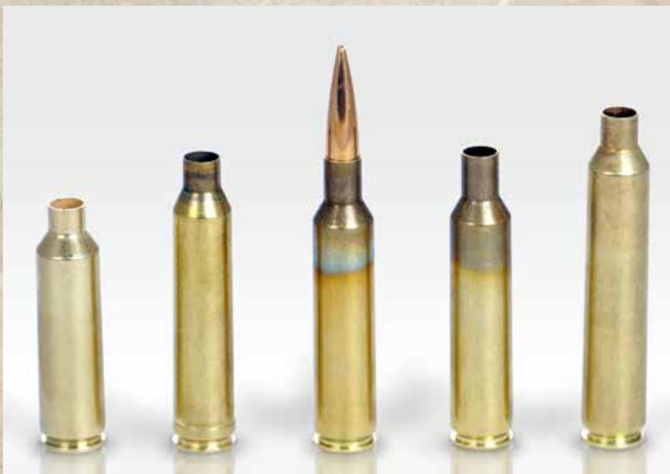
Case comparison: 7WSM, 7mm Rem Mag, Loaded 7LRM, Fired 7LRM, 7RUM
